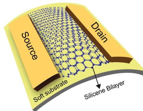
**Fig. 6** Schematic diagram of a possible spin filter or spin generator device generated by using a silicene bilayer placed on a certain flexible substrate. The bending is posed through the soft substrate.
